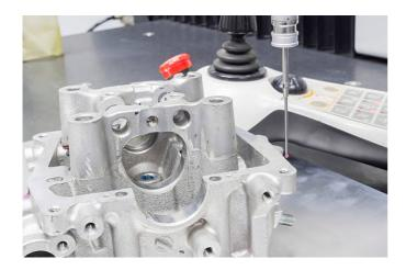
When it comes to form and position tolerances, RapidDirect adheres to a 'K' level by default, in the absence of specific customer requirements.
